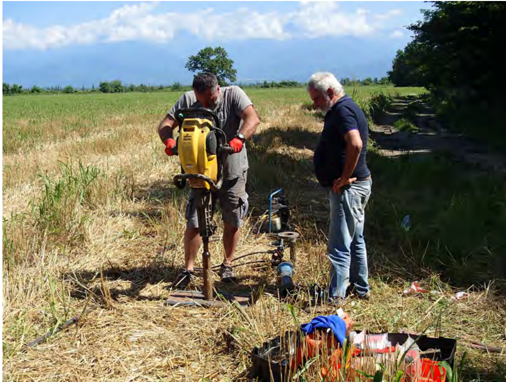
Fig. 6. Levan Navrozashvili drilling core AN_20
