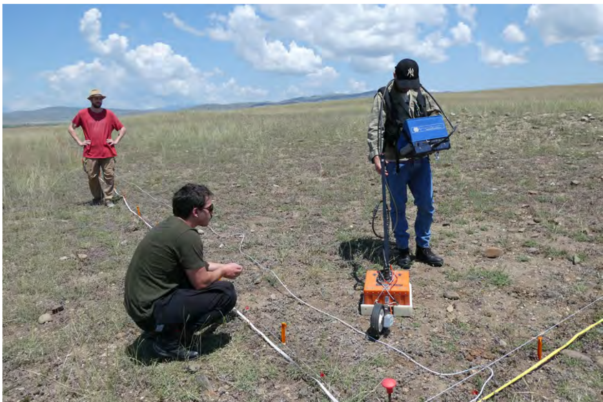
Fig 3. Nika Metreveli and Dimitri Akubardia operating the Ground Penetrating Radar on the Kurgan field
