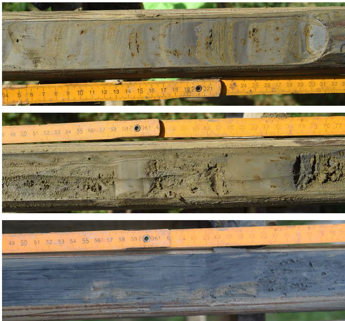
Fig. 13. Jandara Lake, core DR25-A2, depth 2.48-2.77 m, showing low (clay) and high energy (sand) sediments accumulated in river environment (above); core DR25-A2, 3.04-3.33 m, showing alternating laminae and thin layers of clay and silty clay, prevalently oxidised (in the centre) and core DR25-A2 core, depth 4.48-4.77 m; dark grey to blackish clay sediments (below)
