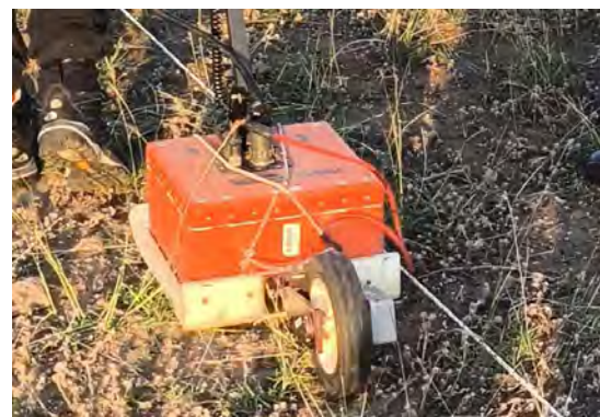
Fig. 14. GSSI SIR-3000 GPR system (left) and 400 MHz antenna (right)
