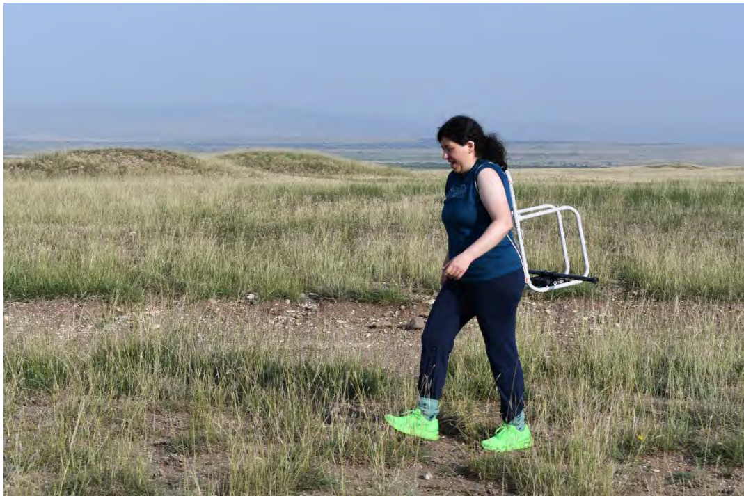
Fig. 7. MagDrone R3 on site positioned on the back of the operators
